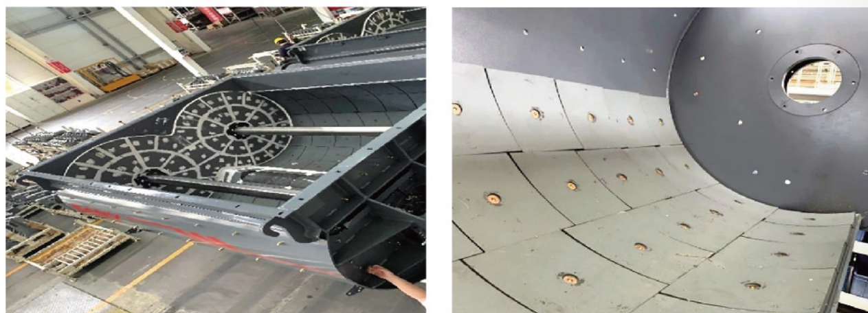
采用超级耐磨钢 NM450SP 制作的水泥搅拌罐衬板 Lining plate in cement mixing tank made of super wear-resistant steel NM450SP
