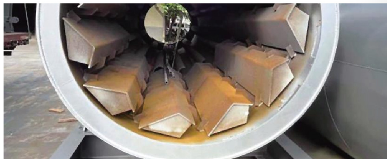
采用耐热耐磨钢 NM450HiTemp制作的叶片:回收料加热筒 Blade made of heat and wear resistant steel NM450HiTemp: recycled material heating drum
