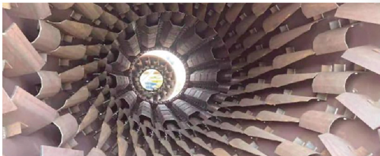
采用耐热耐磨钢 NM450HiTemp制作的叶片:砂石加热滚筒 Blade made of heat and wear resistant steel NM450HiTemp: sand and stone heating drum
